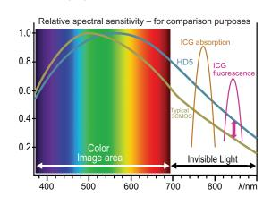
Incorporating Canon's innovative three-chip technology, the IK-HD5 provides approximately 3dB increased sensitivity in the near-infrared spectrum through 700-870 nm. When equipped with the appropriate optics and filters, the IK-HD5 can be used for both visible light and near IR imaging applications such as indocyanine green (ICG) and other fluorescing agents.
