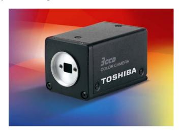
The three chip camera features a 1/3" IT-CCD sensor (410,000 pixels), 570 TV (H) resolution, and an RGB micro prism system to capture accurate, computer-ready color images. With RS-232 serial interface, a 2:1 interlaced scanning system, on-screen menu and C-mount lens flange, the affordable 3CCD camera can be easily integrated into an existing system.
