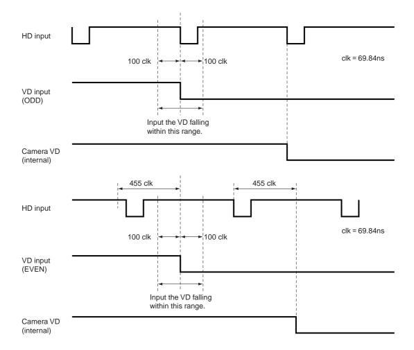
The phase relationship of the external HD and VD should correspond to the center phase (i.e., the external HD falling edge) as illustrated in the above diagram.
