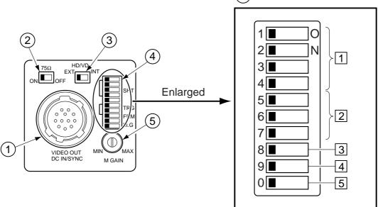
① VIDEO OUT DC IN/SYNC plug (12-pin connector)
