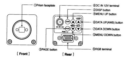
① Prism faceplate The protection cap is attached on the lens mount portion. After removing the
